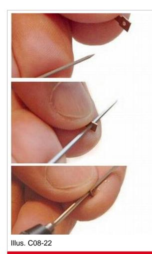
The existing hole in the reed needs to be enlarged to fit the external diameter of the stud bolt (1.4mm).
