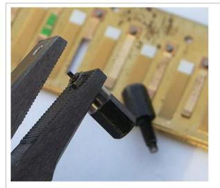
Here the bit 10a for de-riveting has been screwed into the pliers.
