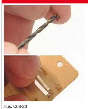
When reaming out the hole, a tiny burr will form on the reed. In order to avoid play at a later point in time between reed and plate, it's necessary to deburr the reed with the Drill Bit (13), using minimal pressure.
